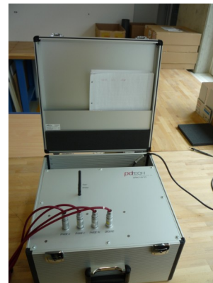
Figure 3: DRA-3 which can perform PDC tests up to 10 kV
